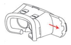
Insert your mobile phone into the holder on the front of the front section. The spring loaded holders will open and close to hold your phone securely.
