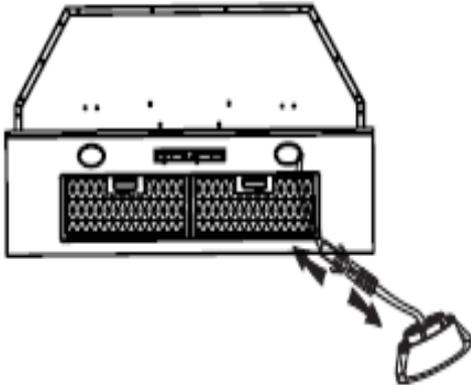
5. Remove the light fitting from the panel by pulling back the 2 spring clips, and carefully push the fitting out of the panel.
