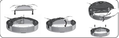
Please put together and take apart the trailing bar assembly according to the above photo. Tips: 1.When installing the snap joint on both sides, either press or take it out carefully at a 900 (degree)angle to the cleaner, to keep the joint in good condition.
