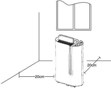
Allow at least 20 cm space around the unit. This dehumidifier is designed only for indoor residential or small office applications and any commercial or industrial use will invalidate the warranty.
