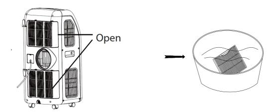
**Please note**: If used, the optional active carbon filter (cloth) should be replaced every 3-6 months based on the environment.
