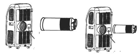
Extend one head of the hose and screw it into the unit anti-clockwise. The hose can be removed by screwing the hose clockwise.
