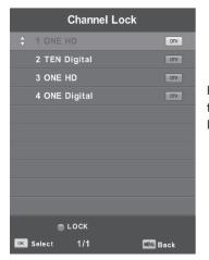
Press  $\mathbf{\nabla}$  /  $\mathbf{\Delta}$  button to select Channel Lock then press Enter button to enter sub-menu to select. Press button to lock or unlock the channel Green .
