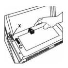
Place the glass under the location bracket (x) in the direction of C.
