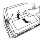
You must remove the oven door glass before cleaning. Push the glass in the direction of B and release from the location bracket (x). Pull the glass out in the direction of A.
