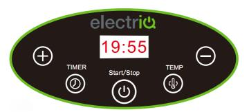
from 35°C to 70°C in 5°C increments. Press the "TIMER" button to set the timer. The timer is selectable with 30 minute increments up to 48 hours. After the timer lapsing fan will continue to run for approximatively 10 more seconds than will go in standby. If the food is dried and timer still working turn off the machine by pressing the "START/STOP" button twice, than unplug it and store it in a safe and dry place.
