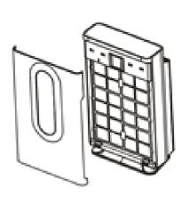
3) Load the composite filter into the front of the unit and replace the cover.
