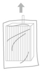
Remove the filter from the plastic protective packaging
